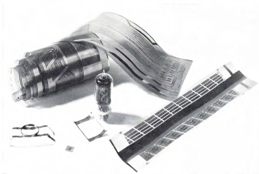
Fig. 12. Some products made by the PD photoplatting process. Right: part of a colour-television delay line. Left, foreground: a microphone diaphragm. Background: strip with conductor pattern that can fulfil the same function as a 'tree' of connecting wires (cable-form) as used in telephone exchanges. Centre: an indicator tube whose anode (lying in front of the tube) is in the form of a thin mesh made by the PD process. The tiny square at the centre of the foreground is an integrated circuit on film with conductor pattern made by the PD process.
