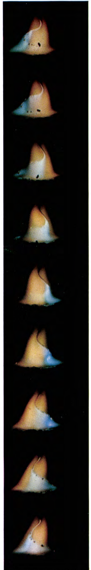
Fig. 5. a) Photograph of the plasma-MIG process with rotating arc. The contours of the surface of the molten wire tip can be seen inside the plasma. b) Series of frames from a high-speed film (4000 frames per second) of the rotating arc.
