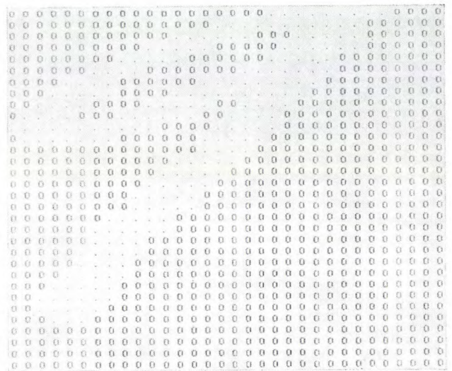
Fig. 13. Matrix with occupied positions (marked with a dot) and unoccupied positions (marked with a zero); the occupied positions represent the numeral nine . In this form the numerals are ready for skeletonization.
